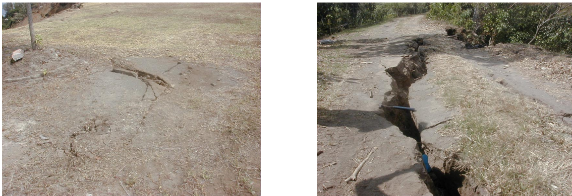
Figure 2.23. Crack at the top terrace (photographed on Jan. 14 by Mr. Jose Antonio Rivas)
