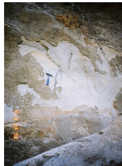
Figure 2.21 Cracks and joints on the exposed intact pumice
