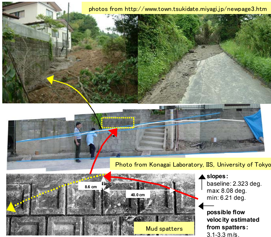
Figure 5. Marks of landslide mass (middle) and spatters (below) remaining on mortar block wall
