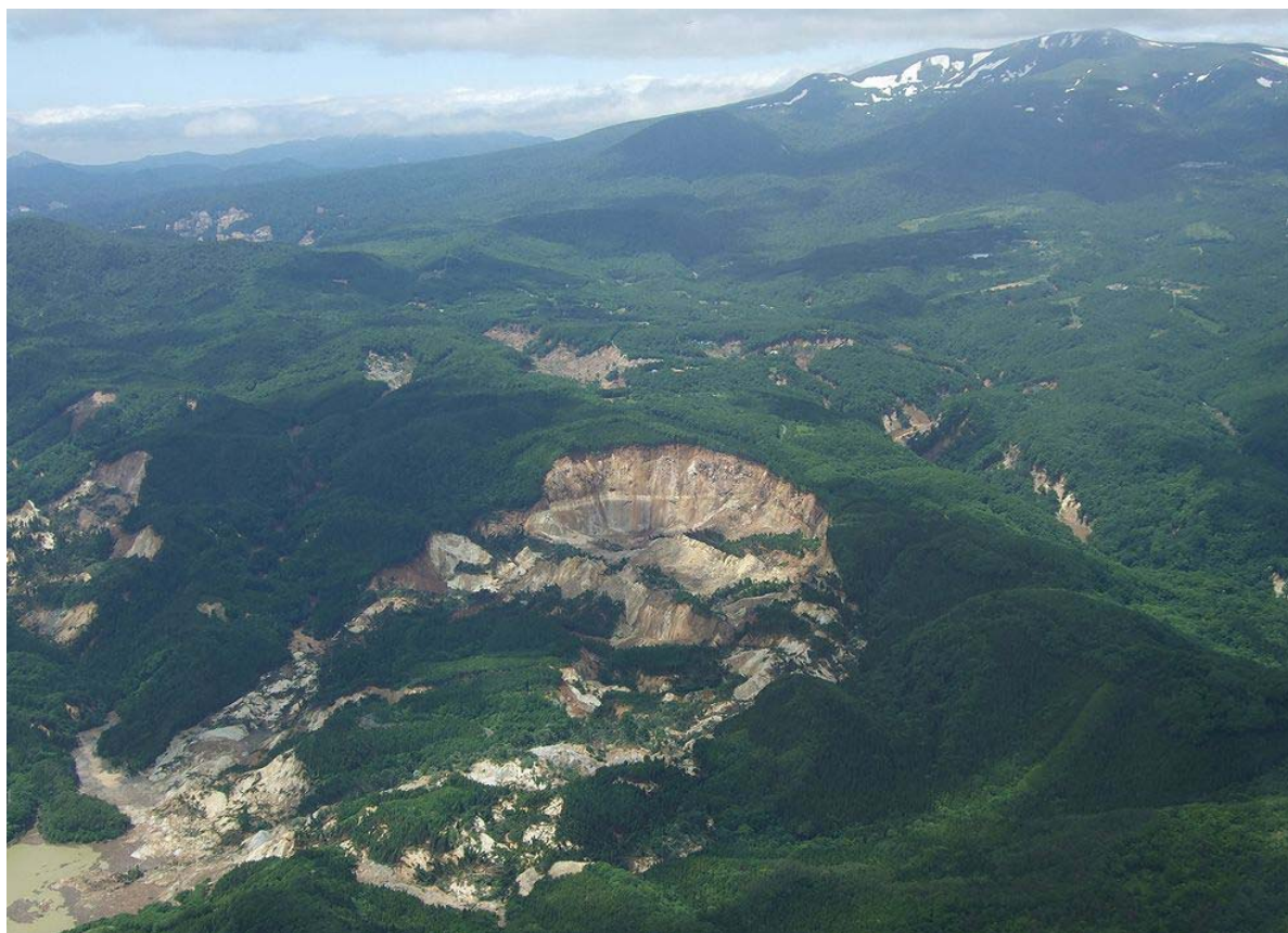
Fig. 1. Landslide at Aratosawa dam: Aerial photo of the largest landslide with Kurikoma Volcano rising behind. The terrain here is suggestive that similar landslides have been reactivated. A wide-spread and almost horizontal laminar structure of loose volcanic sands and ashes is being exposed on the escarpment. When wet, some pieces of light-gray rock fragments taken at the toe of the landslide mass smelled strong hydrogen sulfide (see Fig. 3). (Photo by K. Konagai)
