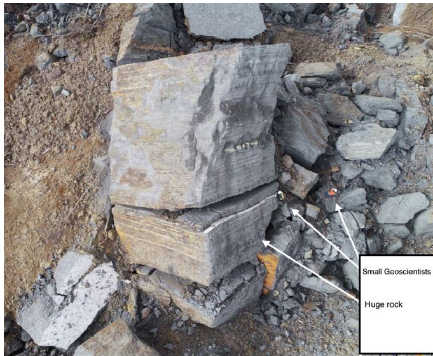
Figure 3-28. Size of blocks in the head scarp of the landslide at Tower 107
