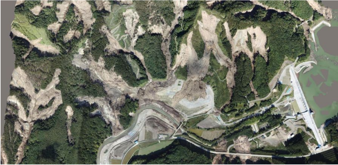
Figure 5-27. Landslides (Scar Areas) Below Lower Atsuma Reservoir (Credit: GEER)
