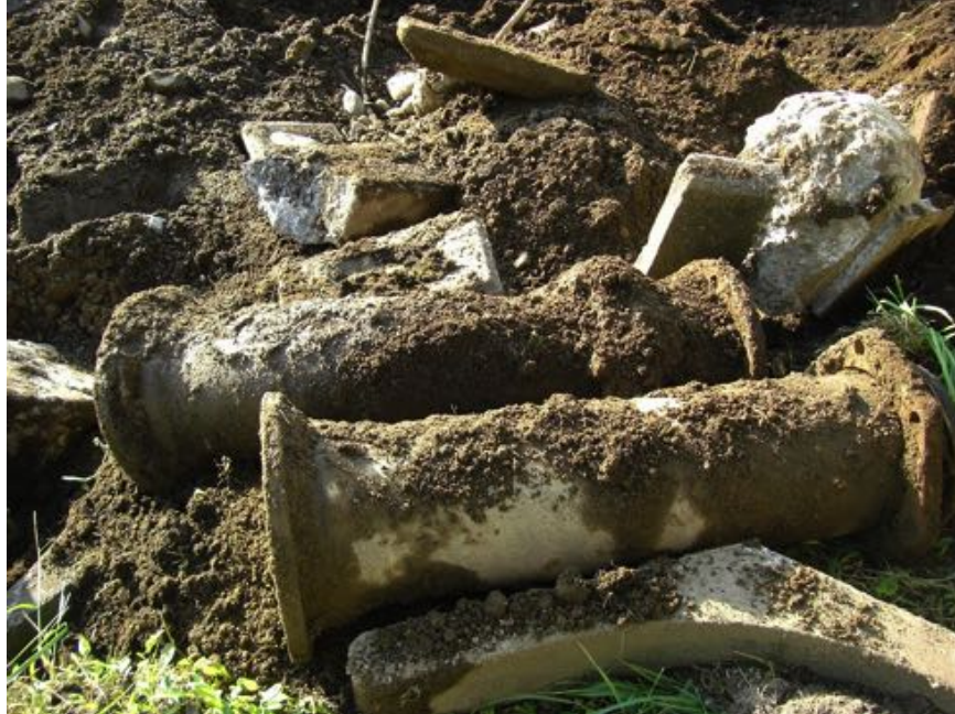
Figure 5-17. Removed Elbows of 200 mm DIP (credit: Kubota)
