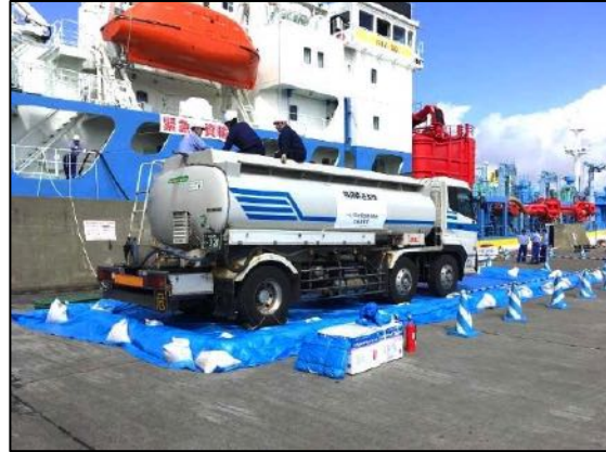
Figure 8-8. Heavy Oil unloading to oil tanker (note oil spill preparation)(Source: MLIT)
